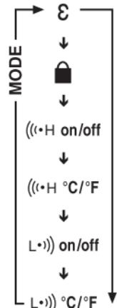
Various functional settings can be applied using the **additional function (mode) selection button** 22. The TP6 switches to the next functional mode each time the mode button is pressed (see illustration).
